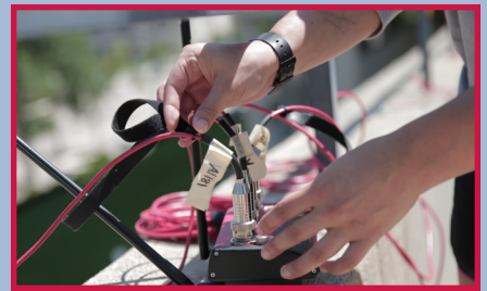
Graduate students attach sensors to the Park Street bridge to collect vibration data.
