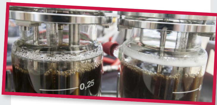
Benchtop bioreactors contain conversion residue from lignocellulosic ethanol production. Photo: Great Lakes Bioenergy Research Center.
