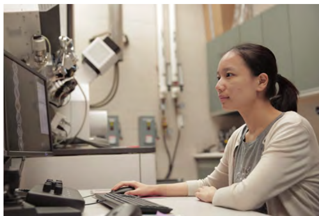
Chemical engineering PhD student Yingxin Guan conducts research with a plasma focused ion beam microscope (pictured in background). The microscope is used for high-speed nanomachining to create test samples for transmission electron microscopy and other experiments.
