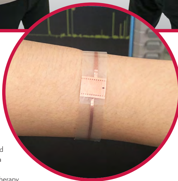
Materials Science and Engineering Professor Xudong Wang fits a new wound dressing around the wrist of graduate student Yin Long. The device stimulates healing using electricity generated from the body's natural motions. Photo: Xudong Wang.
