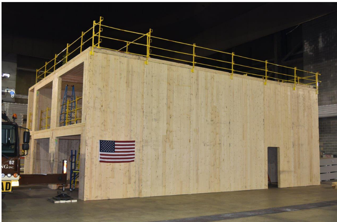
Forest Products Laboratory researchers created five fire scenarios in a two-story, full-scale test building constructed using cross-laminated timber.
