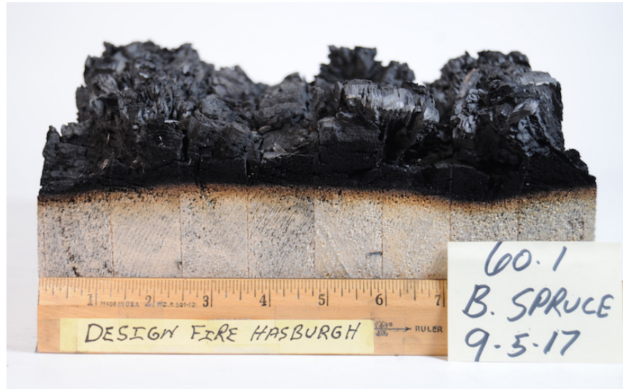
Laura Hasburgh has conducted extensive testing to determine the charring rates of six wood species, including black spruce.
