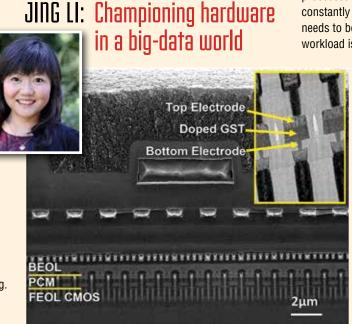
A diagram of one of the innovative computer chips Li is developing.
