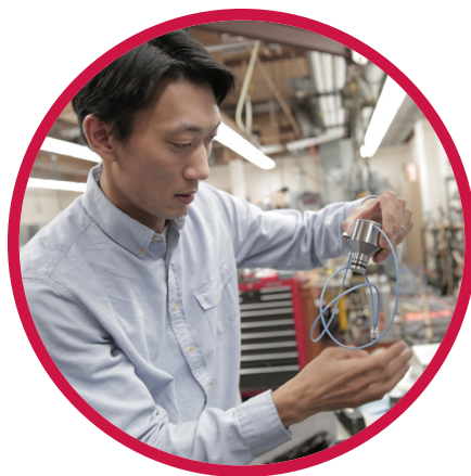
Hiroki Sone prepares a rock sample for deformation measurements under stress conditions in a triaxial rock mechanics apparatus. Photo by Stephanie Precourt.
