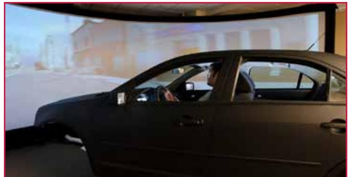
The Driving Simulation Laboratory at UW-Madison includes 270 degrees of virtual simulation, thanks to a 24-foot wraparound screen with computer video projection, audio and car-tracking movements as small as one degree in any direction.
