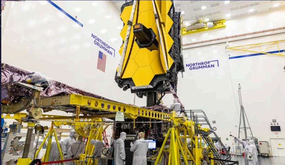
Engineers deploy the forward and aft pallets that hold the James Webb Space Telescope's sunshield during launch as part of Webb's last deployment tests at Northrop Grumman in Redondo Beach, California, in December 2020. Credit: NASA.
