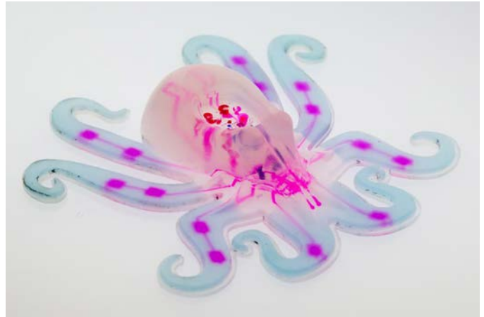
Wehner helped create the world's first autonomous, entirely soft robot, dubbed the Octobot. Credit: Lori Sanders/Harvard University.
