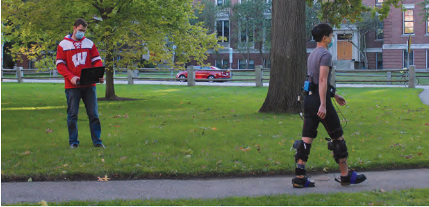
The researchers' unique wearable sensor can help tune exosuit controllers to work effectively for individual users in various environments. Credit: Harvard Biodesign Lab.
