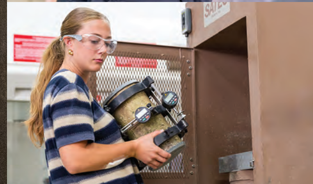
Top: Steven Cramer, a civil and environmental engineering professor emeritus, carries a fractured concrete sample after testing it in a hydraulic press. Cramer oversaw testing of the samples, which were first poured in 1923, to conclude a 100-year study. Bottom: Civil and environmental engineering junior Ella Thomas loads a 100-year-old concrete sample into a hydraulic press for testing. The concrete is wrapped in sensors that measure stresses while the sample is under load. All photos: Alex Holloway.
