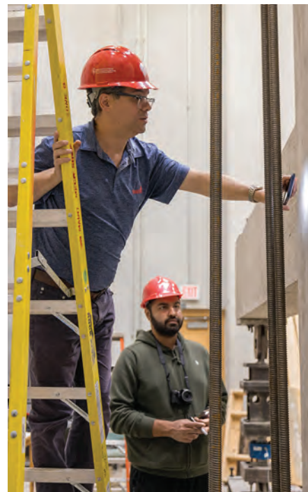
Professor Gustavo Parra-Montesinos looks at where a test column joins a beam during an experiment in the Jun and Sandy Lee Wisconsin Structures and Materials Testing Laboratory. Parra-Montesinos conducted the tests to study proposed code changes to headed rebar insertion depths where concrete columns and beams intersect. Photo: Alex Holloway.
