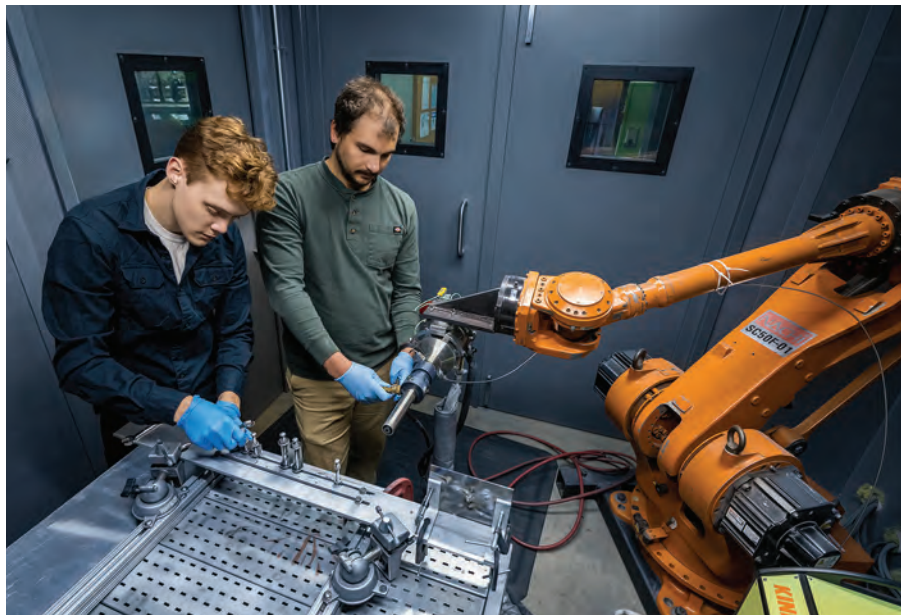
Graduate students Evan Willing (left) and Tyler Dabney set up equipment to apply a coating via cold spray in Professor Kumar Sridharan's Cold Spray Laboratory. Photo: Joel Hallberg.
