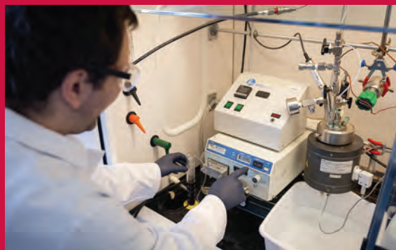
Dillon Hofsommer adjusts a membrane flow bioreactor in his lab at the Wisconsin Energy Institute. Scientists with the Great Lakes Bioenergy Research Center use the reactor to extract valuable aromatic chemicals from lignin, a part of plant cells often treated as waste. Photo: Chelsea Mamott/Wisconsin Energy Institute
