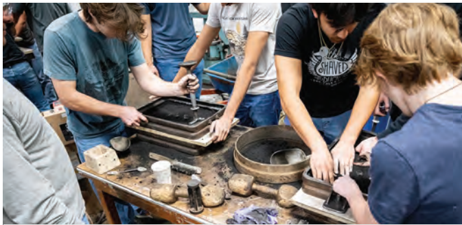
Students compact sand around a model to create the mold cavity for a screwdriver handle. Photo: Sarah Maughan/UW-Madison.
