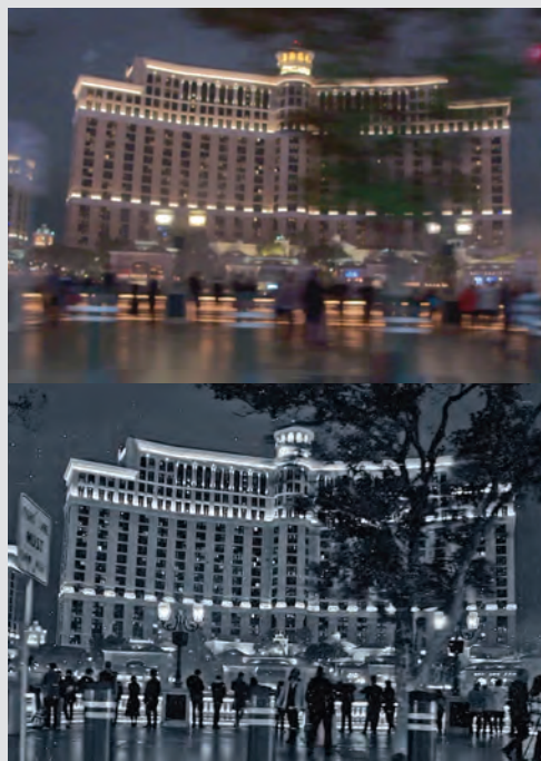
On the top is an image taken on the Las Vegas strip with a high-end automotive camera, while on the bottom Ubicept's hardware and software is leveraged to reduce blur and noise and deliver a clear image. Image courtesy of Ubicept.
