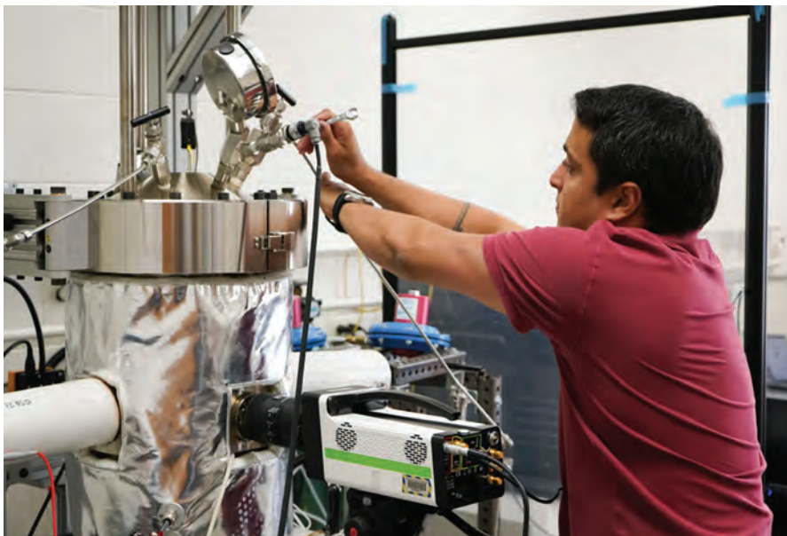
To study critical heat flux, PhD student Bruno Serrao sets up his custom pool boiling experiment to monitor how material surface characteristics impact heat transfer. Photo: Lili Sarajian.
